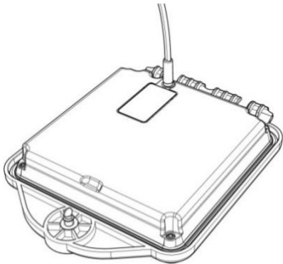
Figure 4.13 Charging the transmitter Li-Ion battery pack
