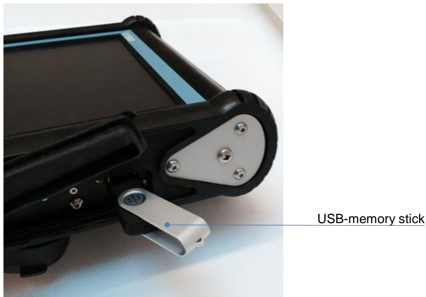
Figure 10-1: Insert a USB memory stick into the USB port on the Display Unit to export data.
