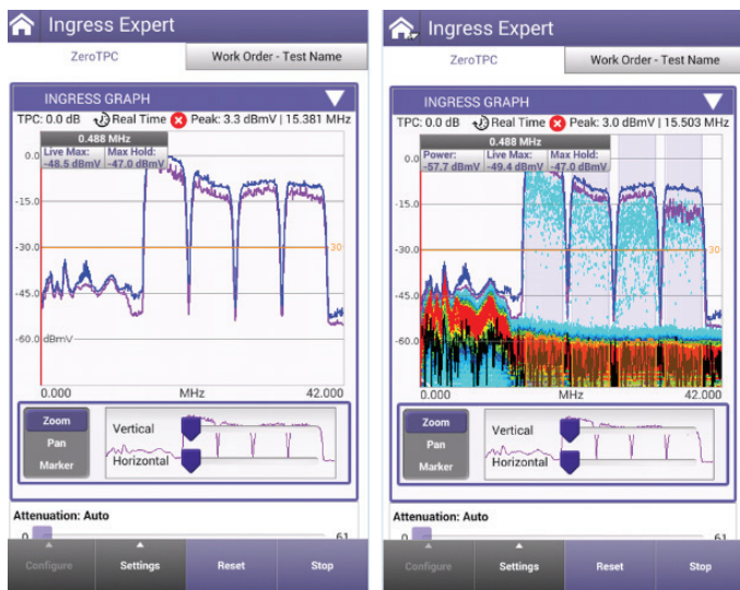
Live upstream carriers normal spectrum analyzer type view
