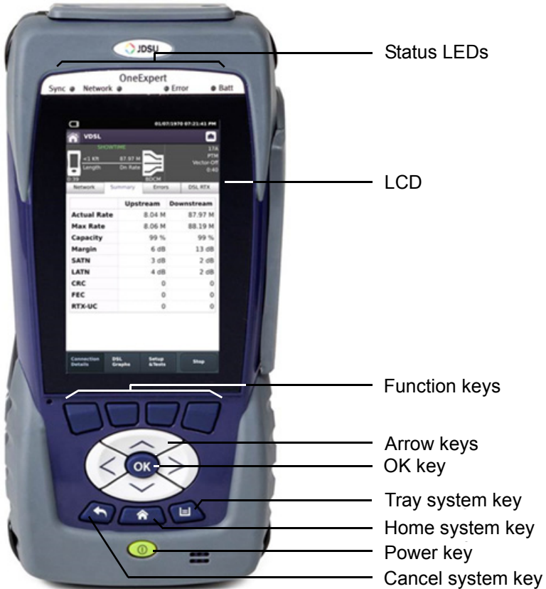
Figure 3 OneExpert DSL front panel
