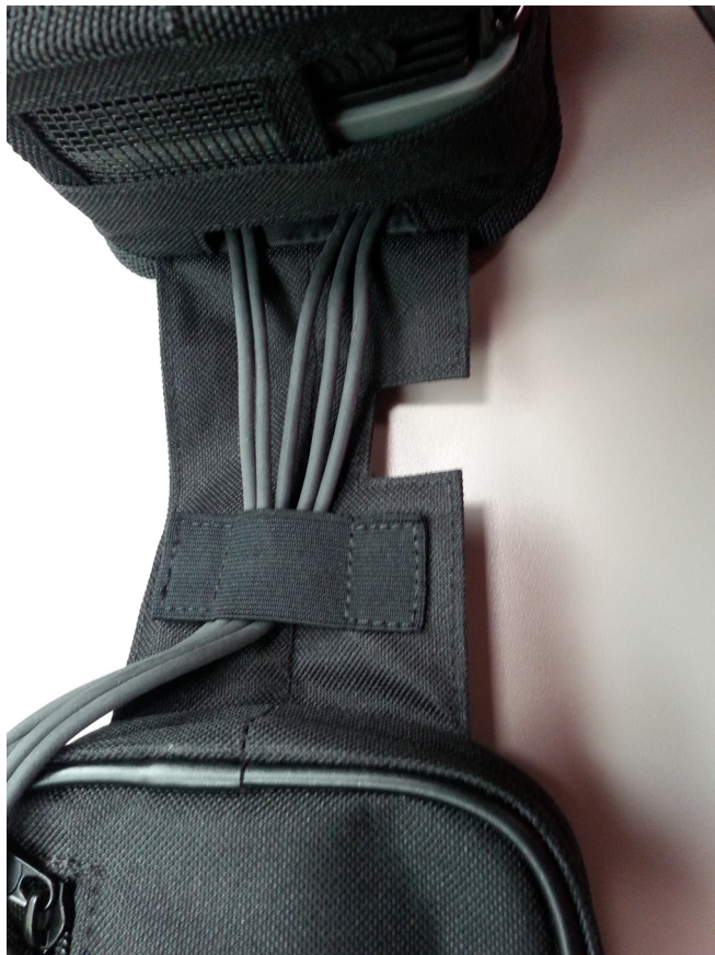
Figure 15 Cable routing through the hinge of the glove
