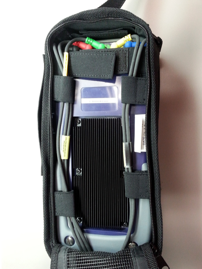
Figure 14 Cable routing through the back of the glove
